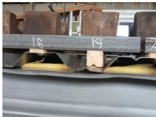
Figure 5 – Loss of stability of the compressed narrow flange of the cassette profile of the edge zone of the panel and the destruction of the blind rivet joint. Loading stage 6
