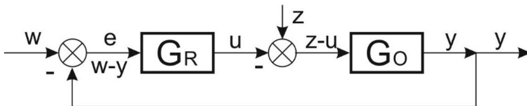
Fig. 1. Scheme of the simplified aircraft engines automatic control system, where:  $G_R$  – controller transfer function,  $G_O$  – object transfer function,  $w$  – input signal delivered by the engine control lever,  $z$  – input signal (disturbances),  $y$  – output signal (engine rotational speed),  $e=w-y$  – input signal for the controller,  $u$  – output signal from the controller. [2]
