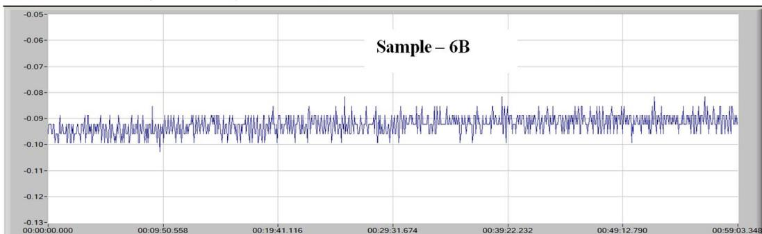
**Figure 19** – Diagram of the dependence of friction coefficients on time: sample – 6B
