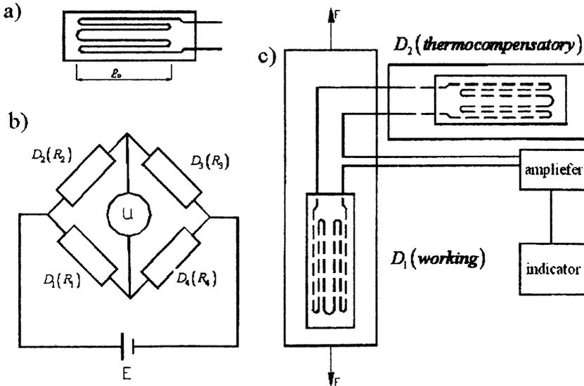
Fig. 1.4. Scheme of the electrical resistance strain gauge
