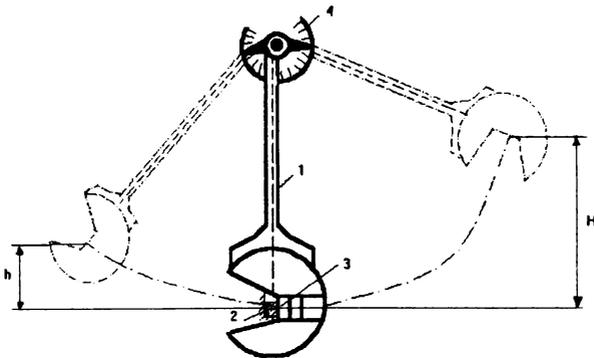
*1 – pendulum, 2 – sample, 3 – peen (knife), 4 – scale of measurements*
