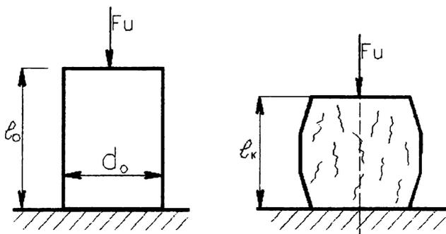
*Fig. 4.5. Nature of destruction of a brittle sample*
