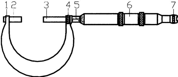
1 – a bracket, 2 – a heel, 3 – a micrometer screw, 4 – a stopper,
