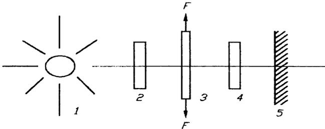
1 – light source; 2 – polarizer; 3 – model; 4 – analyzer; 5 – screen
