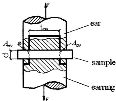
*Fig. 5.1. Device for testing of metal for a cut*
