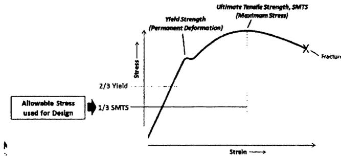
Fig. 2.6. Diagram of Allowable Stress Design (ASD) reckoning
