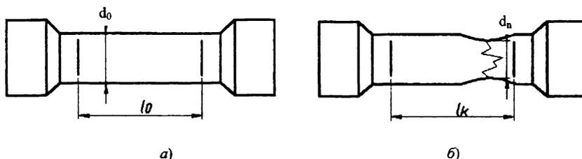
*a) sample for testing of metals at stretching; b) the shape of destruction of a ductile material sample*
