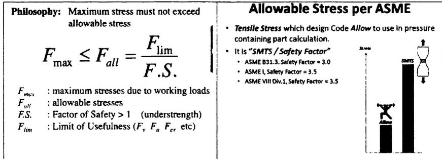
Fig. 2.5. Calculation of Allowable Stress Design (ASD)
