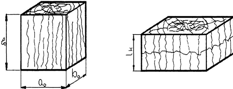
**Fig. 4.7. The nature of destruction of a timber cube at compression along fibers**
