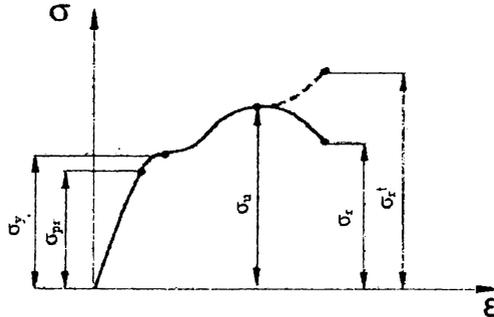
Fig. 2.5. Diagram of engineering stress
