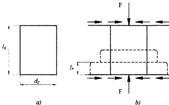
**Fig. 4.1. Friction forces at compression of sample**
