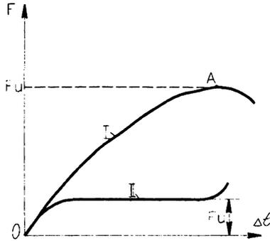
**Fig. 4.6. Diagram of compression of a timber**
