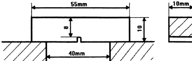
**Fig. 8.3. Standard samples for shock test**
