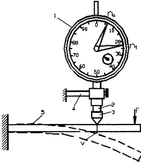
1 – frame with a scale, 2 – contact rod, 3 – head, 4 – support, 5 – part (construction)
