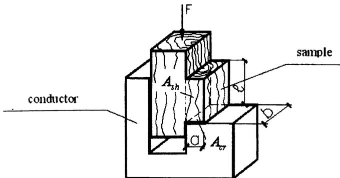
*Fig. 5.2. The device and the sample for testing of a timber for shearing*
