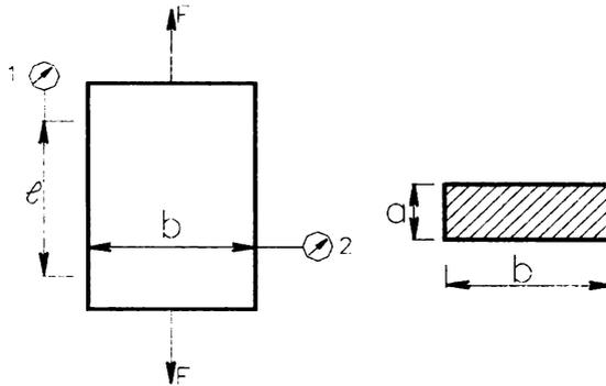
**Fig. 3.2. Sizes of a sample**
