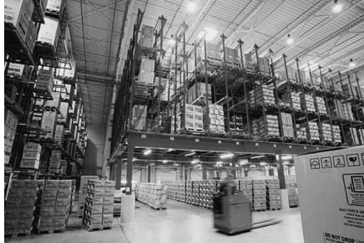
Figure 23 Shuttle racking above despatch bays (courtesy of Toyota)
