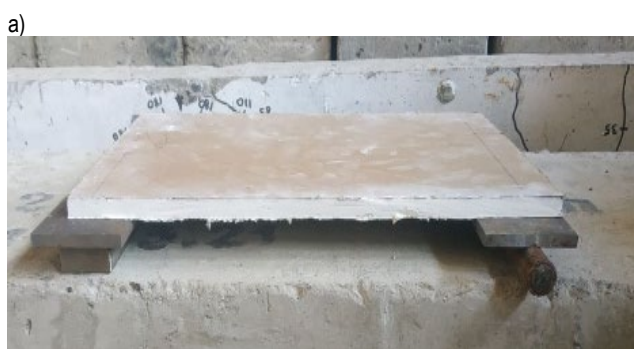
a) location of the slab on supports located at a distance of 350 mm; b) destruction of the slab under load applied in the middle of the span
