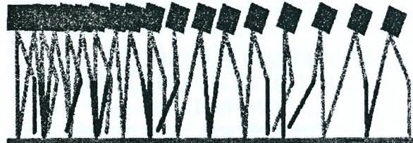
Fig. 12 – Stick diagram showing a walking sequence of the biped robot with increasing average velocity increases.
