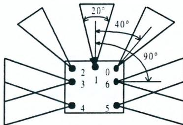
Fig. 2. Ultrasonic sensors configuration
