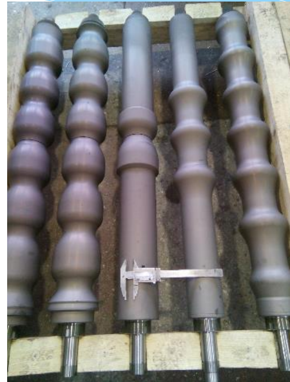
Shafts for the manufacture of metal tiles
