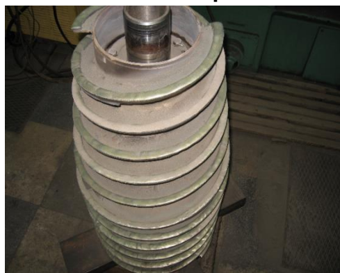
Shaft of compressor
