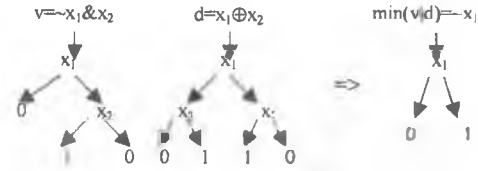
Figure 1: Minimization operation on BDDs, an example
