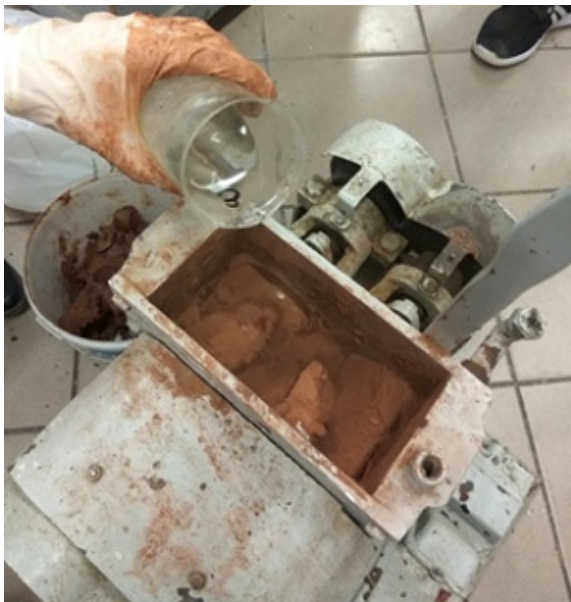
Figure 1. Mixer used to mix ingredients into a ceramic mass (Source: 4)
