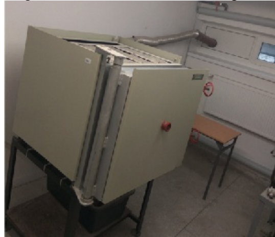
Figure 4. Burn furnace for construction products (Source: 4)
