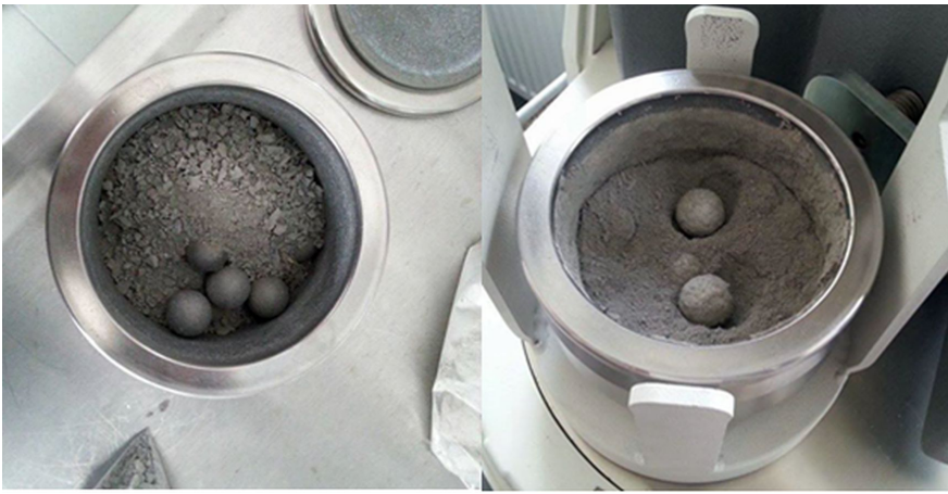
Figure 1. The milling process of preparing recycled binder.
