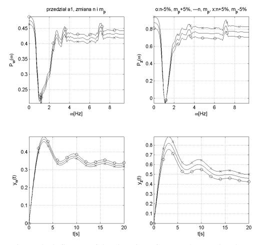
sented the obtained signal waveform for simultaneous n and mp change by 5%.
