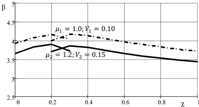
**Figure 4.** Values of the reliability index for a reinforced concrete element under bending with the reinforcement ratio 1 % for various statistical parameters for a probabilistic description of the uncertainties in the bending resistance model
