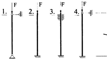
Figure 3.1 – Schemes of fixing column
