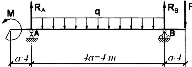
Figure 1.3 – Design diagram of beam and load
