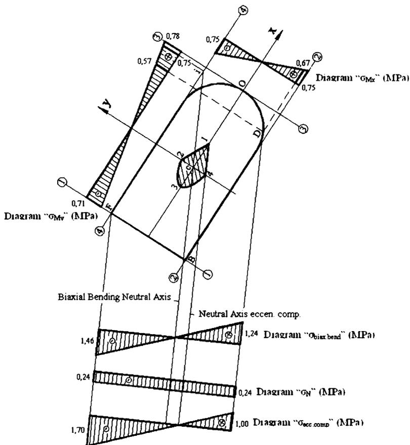
Figure 2.3 – Stress diagrams. Core of cross-section
