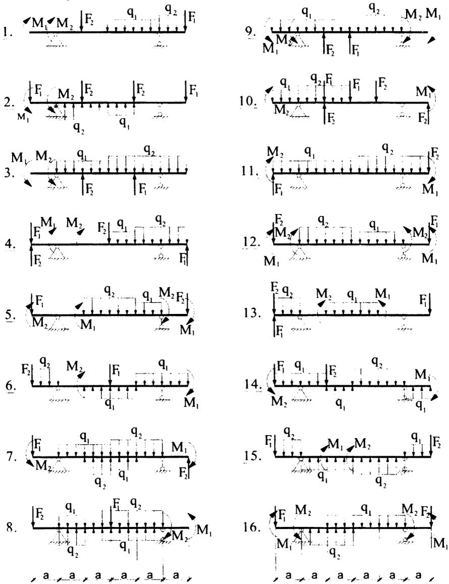
Figure 1.2 – Schemes of beams
