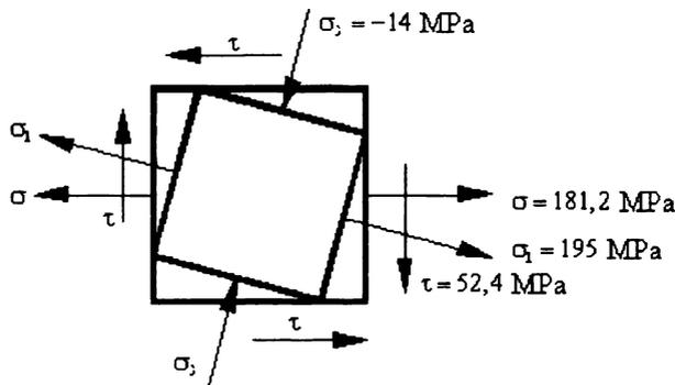
Figure 1.6 – Stress condition in point 2
