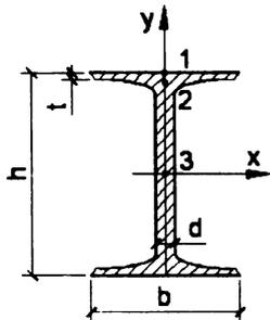
$$\begin{aligned} h &= 22 \text{ cm}; \\ b &= 12 \text{ cm}; \\ t &= 0,89 \text{ cm}; \\ d &= 0,54 \text{ cm}; \\ I_x &= 2790 \text{ cm}^4; \\ W_x &= 254 \text{ cm}^3; \\ S_{x,\max}^{cut} &= 143 \text{ cm}^3. \end{aligned}$$
