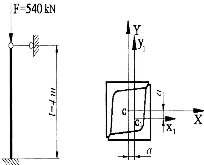
Figure 3.3 – Design diagram of the strut and its cross section
