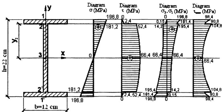
**Figure 1.8 – Diagrams of stresses in section A (on the right)**
