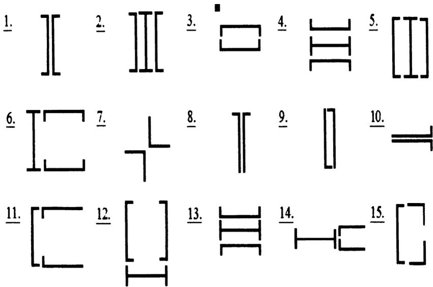
Figure 3.2 – Schemes of transverse sections of composite columns
