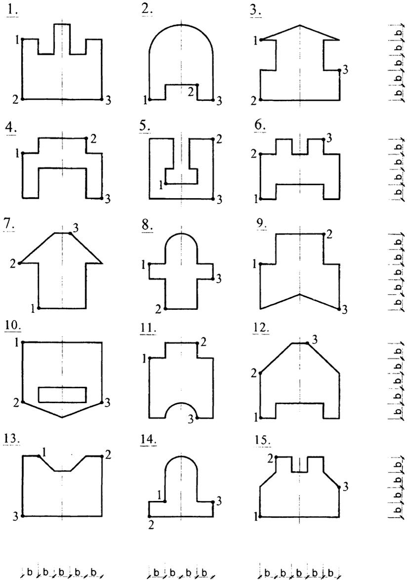
**Figure 2.1 – Schemes of transverse sections of the column with points of application of force**
