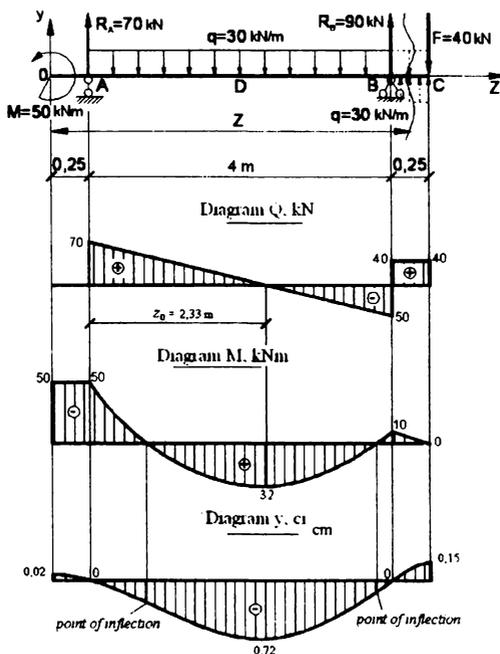
Figure 1.5 – Diagrams of shear forces, the bending moments, deflections
