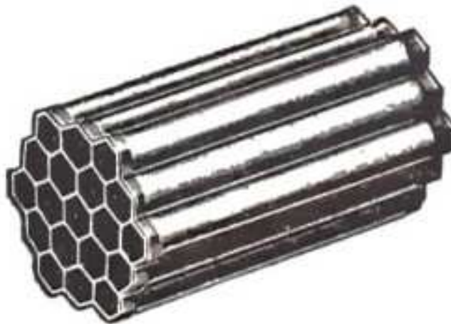
Fig.1 Maybach’s honeycomb radiator
