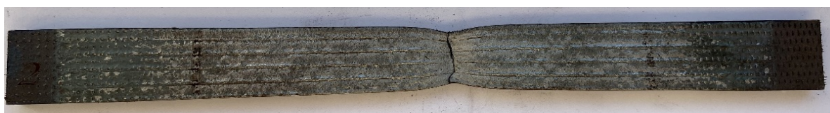
c – destroyed samples (sample 1b)
