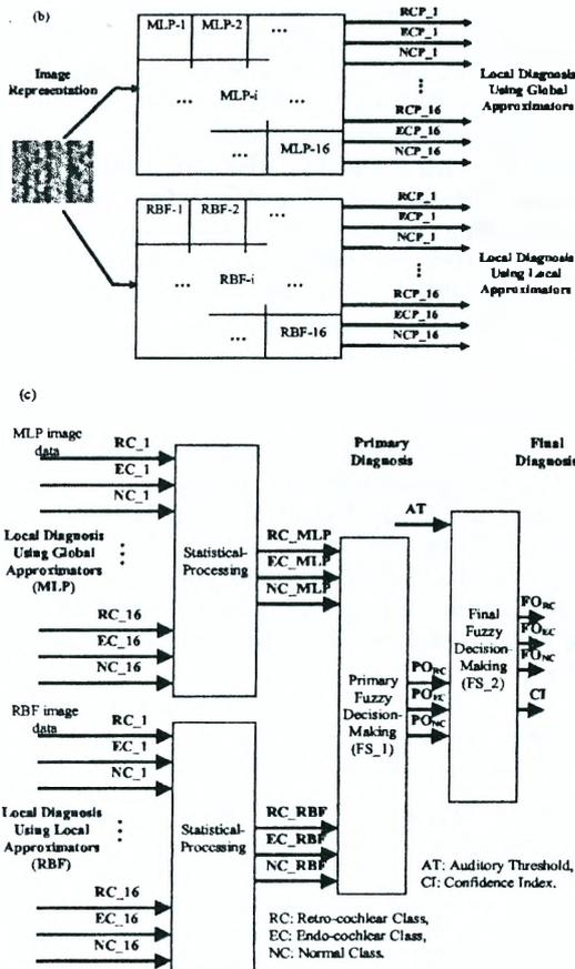
Fig. 4. (a) Image splitting principle, (b) modular neural network architecture, and (c) hybrid intelligent diagnosis synopsis.
