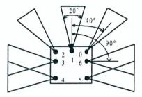
Fig. 2. Ultrasonic sensors configuration
