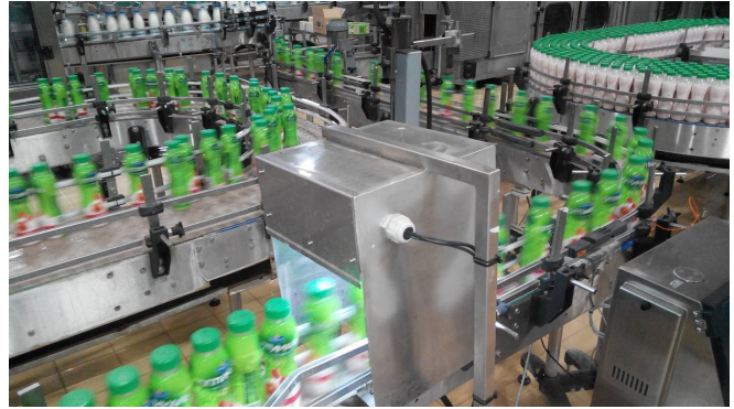
Figure 2. Production line with the camera unit
