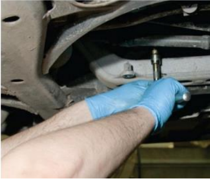
Fig. 1 – Wear nitrile gloves to reduce hand contamination when draining used engine oils
