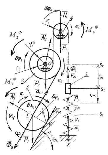
Figure 3 – Rated scheme of the mechanism
