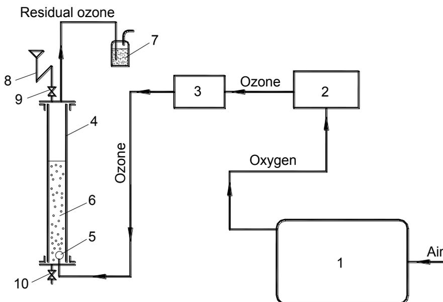
Figure 2. - Scheme of the device for obtaining an ozone solution in distilled water.
