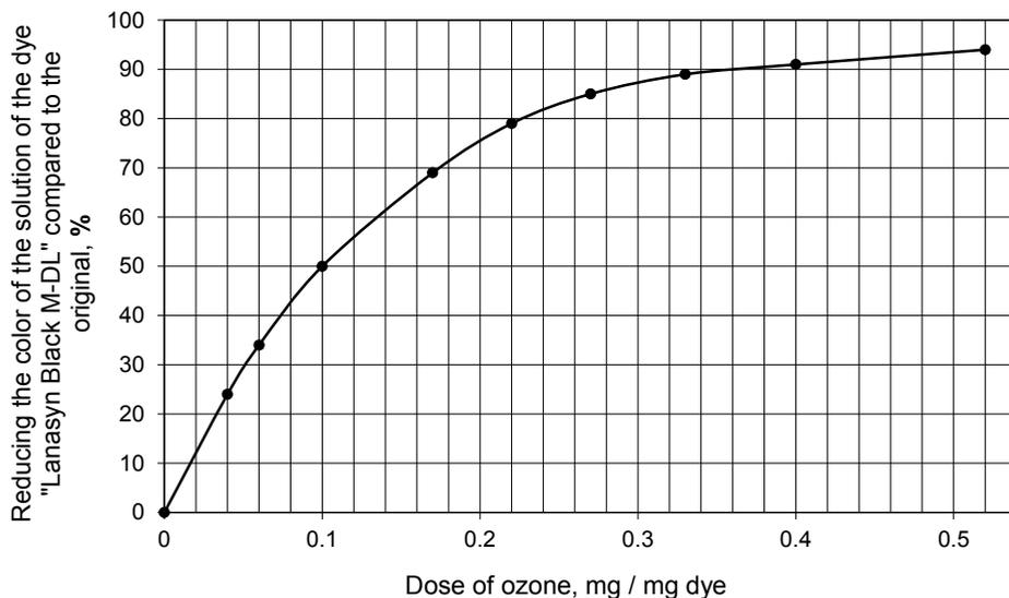
Figure 4. - The effect of the specific dose of ozone on the decrease in the color intensity of the "Lanasyn Black M-DL" dye solution.
