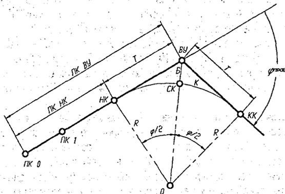
$$\left. \begin{aligned} T &= R \cdot \operatorname{tg} \frac{\varphi}{2} \\ K &= \frac{\pi R \varphi}{180^\circ} \end{aligned} \right\} (4.1)$$
