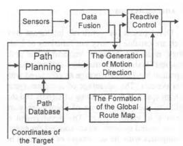
Figure 1. The Control System architecture
