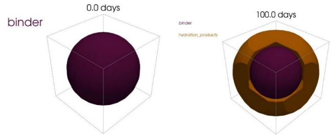
Figure 3 – The evolution of unit cell geometry for BC (The estimated percolation threshold \alpha_{per} = 0,06 )
